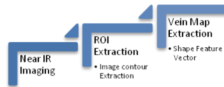
Figure 2: Block diagram of the personal authentication using near IR hand vein images.
